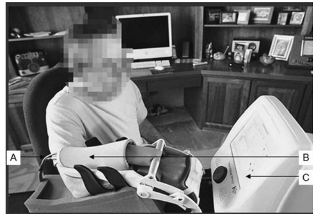
Figure 1. Illustration of the Hand Mentor Pro robotic device and its components. A, Pneumatic hose and data cable; B, arm unit with pneumatic actuator; and C, control box and touch-screen display
