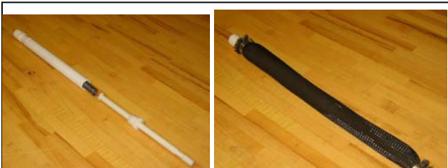
Figure 3. Pneumatic muscles with a spring inside to provide pushing force. The spring parameters are adjustable by changing the resting length.
